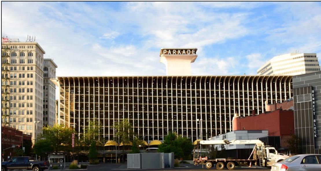
skywalk. Corresponding to the ground floor arched bays, the 52 concrete columns dividing the arched bays of the ground floor are aligned with every fourth column extending upwards from the second story level.
